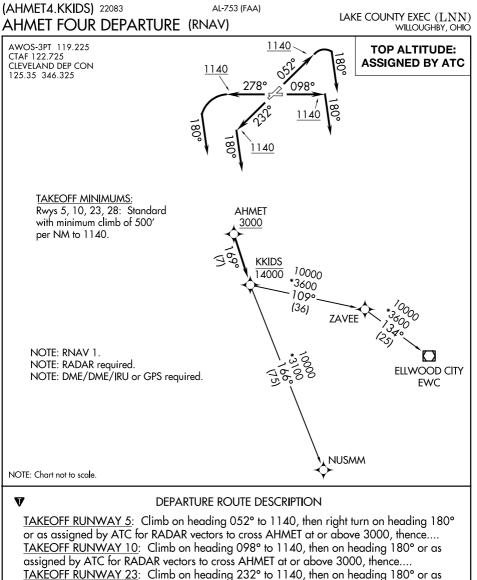
assigned by ATC for RADAR vectors to cross AHMET at or above 3000, thence.... TAKEOFF RUNWAY 28: Climb on heading 278° to 1140, then left turn on heading 180° or as assigned by ATC for RADAR vectors to cross AHMET at or above 3000, thence....
