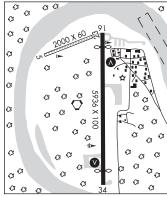
Wx bin fac on arpt, see inside back cover for ops details. Lock wheeled turns NA. Arpt sand Irgr gradation than FAA remdd/See AC150/5200–30. Cold temperature airport. Altitude correction required at or below –46C.
