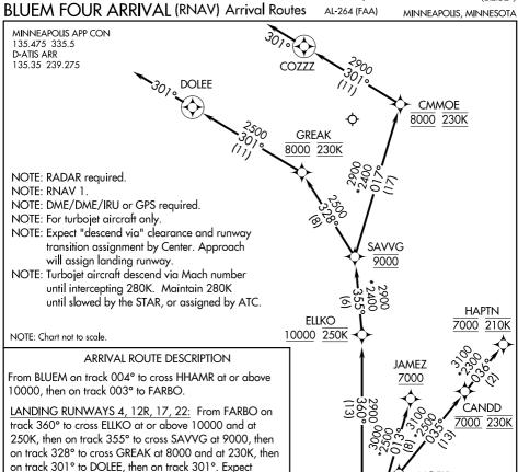
LANDING RUNWAY 12L: From FARBO on track 360° to cross ELLKO at or above 10000 and at 250K, then on track 355° to cross SAVVG at 9000, then on track 017° to cross CMMOE at 8000 and at 230K, then on track 301° to COZZZ, then on track 301°. Expect RADAR vectors to final approach course.
