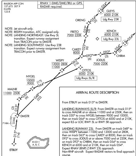
on track 023° to ORENG, then on track 054° to cross GLEYS at 6000 and at 210K, then on track 054°. Expect RNAV (RNP) Z RWY 23R approach. Non-RNP aircraft: Expect RADAR vectors to final approach course. NOTE: Chart not to scale.
