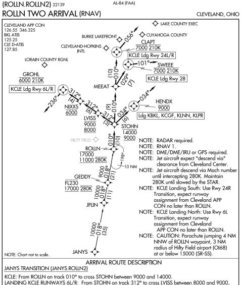
LANDING KCLE RUNWAYS 6L/R: From STOHN on track 312° to cross LVISS between 8000 and 9000, then on track 312° to cross NIXXS at 6000, then on track 312° to cross GROHL at 6000 and at 210K, then on heading 236° or as assigned by ATC. Expect ILS, RNAV (RNP), or RNAV (GPS) approach from GROHL, or RADAR vectors to final approach course.
