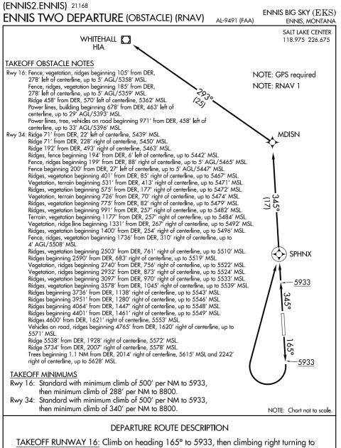
8800 direct SPHNX, thence . . . . TAKEOFF RUNWAY 34: Climb on heading 345° to 5933, then direct SPHNX, thence . . . .
