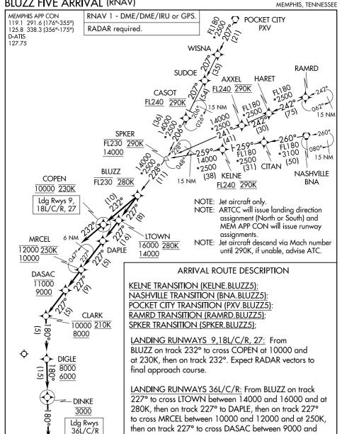
11000, then on track 227° to cross CLARK between 8000 and 10000 and at 210K, then on track 180° to cross DIGLE between 6000 and 8000, then on track 180° to cross DINKE at 3000, then on track 180°. Expect
