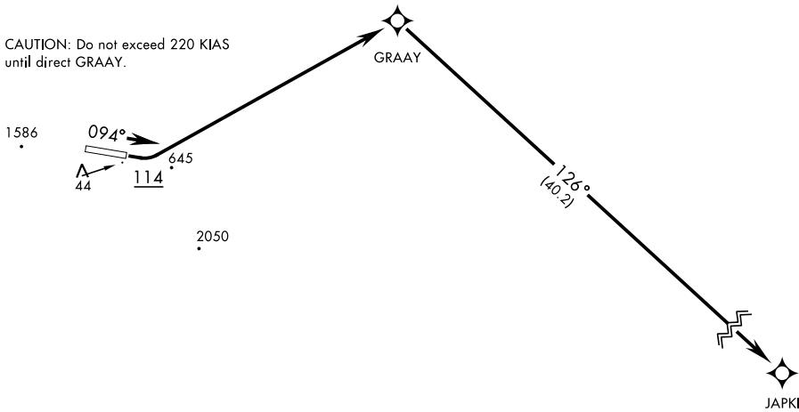
WARNING: High terrain within 2 NM of departure end of runway. Prompt compliance with departure instructions is essential to flight safety. Do not delay initial turn at 114°.
