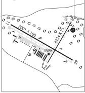
02–20. No ASR coverage blo 10,000′ over KTRK. Special Hazard: Mountainous terrain surrounds arpt and rwys, expect windsheer and downdrafts. Rwy 20 and Rwy 11 distance to go markers installed on left side. Cold temperature airport. Altitude correction required at or below –18C. NOTE: See Special Notices—Glider/Soaring Activities Around the Reno–Tahoe International Airport. Ldng fee.
